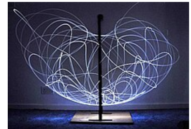
Long exposure of double pendulum exhibiting chaotic motion
